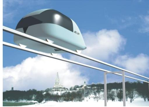
**Fig. 4. Medium-speed single-track SkyWay, speed – up to 250 km/h**
