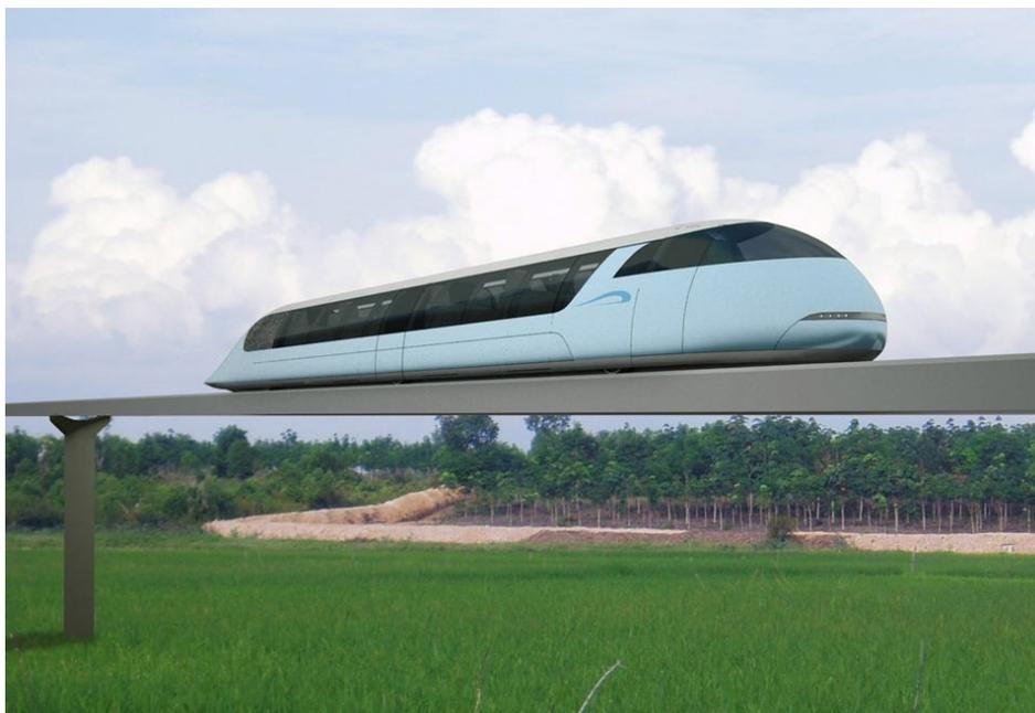
**Fig. 26. Passenger high-speed unibus (capacity – 36 passengers, design travel speed – 360 km/h)**
